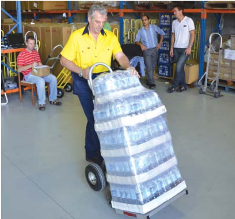
Both the standard hand truck and the Rotatruck Self Supporting Hand Truck were rotated through 360°, while in a relatively vertical position (Figure 28).
