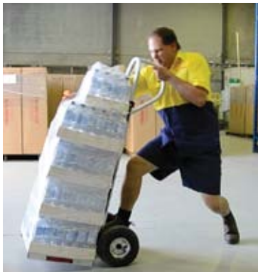
Figure 6 - Pull back load using the standard hand truck
