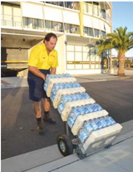
Figure 16 - Negotiating a curb using the Rotatruck
