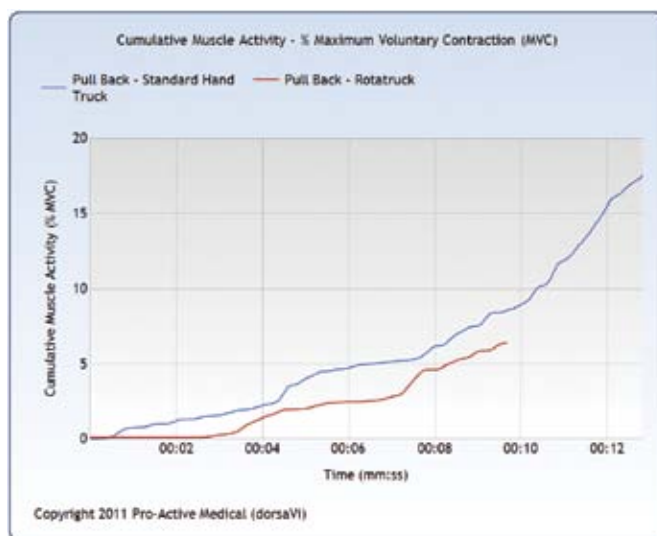
Figure 10 - Comparison of cumulative muscle activity for load pull back
