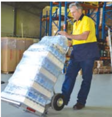
Figure 7 - Pull back load using the Rotatruck self-supporting hand truck
