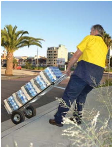
Figure 15 - Curb Negotiation using the standard hand truck to pull load up a curb
