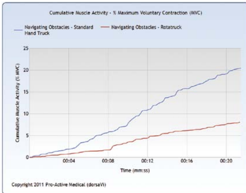
Figure 27 - Cumulative muscle activity comparison of Rotatruck to standard hand truck for navigating obstacles
