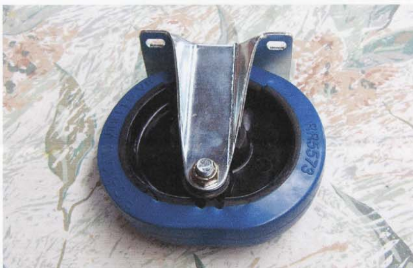
Figure 4 – Competitor's wheel after two drops
