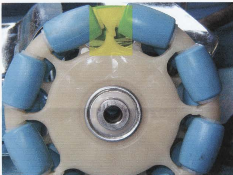
Figure 3 – Rotarola wheel after three drops (Damaged area highlighted)
