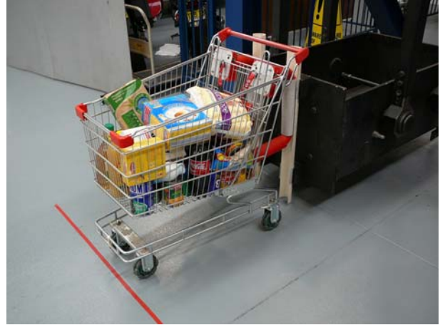
Speed Control Testing - Rotacaster Wheels with Full Grocery Load
