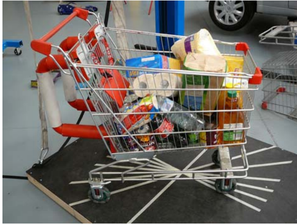
Incline Behaviour Testing - Rotacaster Wheels with 45kg Grocery Load
