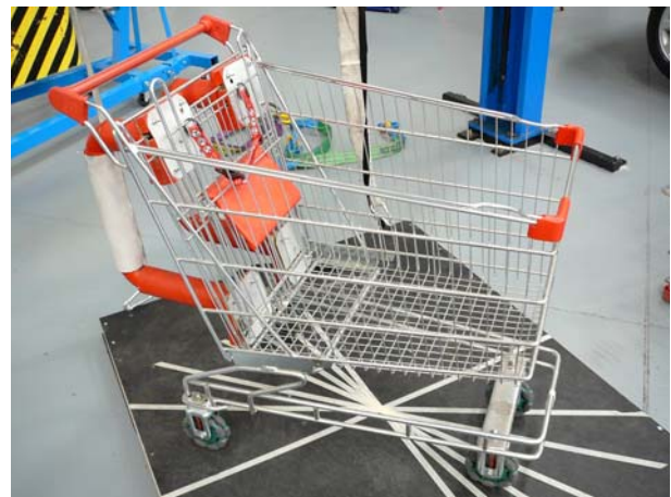
Incline Behaviour Testing - Rotacaster Wheels with No Grocery Load
